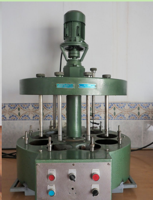
Miniature olive oil mill for EVOO production demonstrations (photo by Juan Carlos Muñoz Flores)
